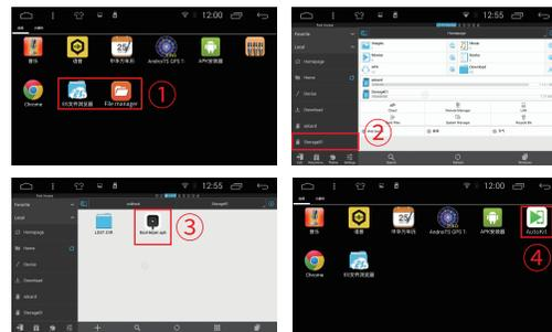
① Plug in the car and wait for the U disk mode to appear on the screen, then open the ES file browser or file manager ② Pop up (storage01) to install and download the APK ③ Click to open the installation ④ The installation is complete
