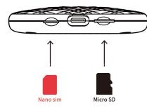
Note: Don't insert the SIM card backward. the wrong way will damage the product's card slot.
